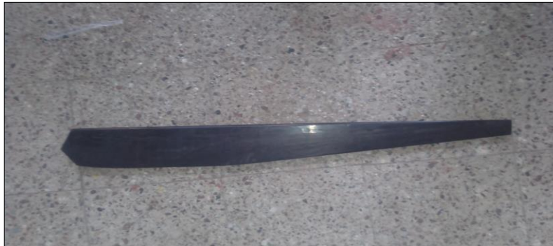
Fig. Polypropylene plastic material blade
