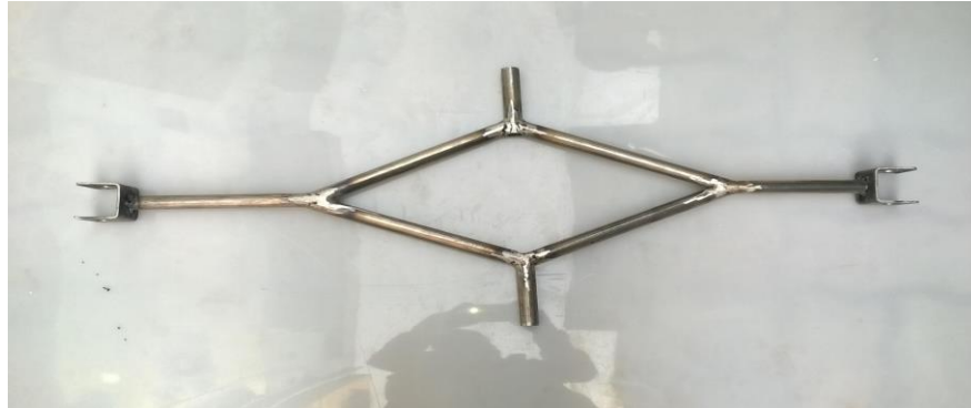
Fig. Sew-saw mechanism
